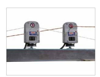
External piezo sensors for multiple yarn insertions. The multi yarn sensor system can control a combination of up to eight wefts divided between up to four weft-feeders at the same time.
