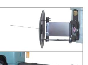
The traditional Leaf brake system is very versatile for applying tension to a yarn, and covers most yarns used today. Our specific recommendation is for high twist yarns, stiff yarns and heavy yarns.
