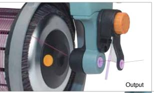
A compensator is used when the yarn needs to be stretched before weft-insertion. A compensator can be used for most yarns, but is mainly used for twist yarns. There are versions for mounting on both the input and output sides of a weft-feeder. Combinations of leaf brake assemblies fitted with compensators are available.
