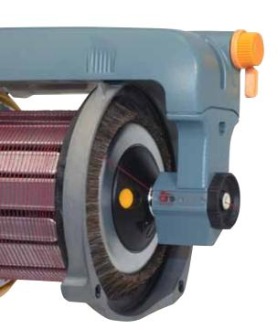
A compensating tensioner for mid/low speeds, that is suitable for most yarns, but particularly suited to give excellent results with endless filament yarns. Has a high wear resistance. And is a selfcleaning unit. With a ceramic version for extreme wear conditions.
