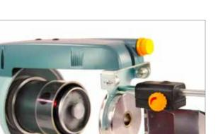
The Low Twist unit is essentially an unrolling device, using an optical system to achieve that the rotation of the package is synchronized with the insertion speed of the loom.
