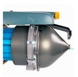
This item can be supplied when the combination of the weight of the yarn together with the insertion rate (meter per minute) of the weaving machine requires that the balloon created by the yarn is correctly controlled. These are for extreme applications and are needed to ensure the yarn can be inserted correctly into the weaving machine.
