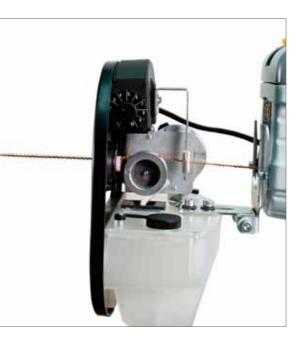
The X2/X3 powered weft lubricator is an automatically controlled oil dispensing device for use on all X2/X3 series feeders. The Oiler is integrated into the systems communications network and is therefore fully synchronized with the feeder's insertion speed.
