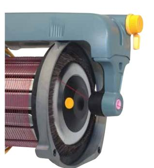
The traditional brush element used for balloon control when the yarn is inserted into the weaving machine, exists in many different versions, including: Direction orientated bristles for the optimum performance, different bristle materials and a range of bristle thicknesses.
