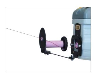
The Twine-Around Brake is used for yarns which have a twist greater than 2000 turns/meter (crepe, silk, viscose, etc.), and where snarls may form during yarn movement.
